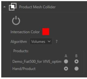
Here the **Product Mesh Collider** is set up with a red intersection using the intersection algorithm **Volumes**.
