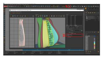
In Shaper, you access the Unfolding Workshop (1.) and then choose which of the 3 methods of unfolding you want to use (2.): One click, Multi-constraints or Follow Boundary. After selecting the method, you can simply click on your model where you want to place controls and see the unfolding on the left side of the viewport. You can then move the control points to adjust the unfolding.
