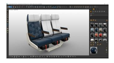
The tools in Patchwork 3D are designed to ease the workflow. The unfolding tool, with it's «one click technique», is great to quickly unfold your surfaces and create uv mappings.
