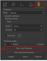
In Shaper, you can quickly create an illumination for your model by opening the lighting tab (1.) and adding lights to an illumination layer.
