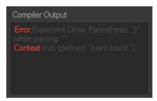
Compiler output error for missing final parenthesis.
