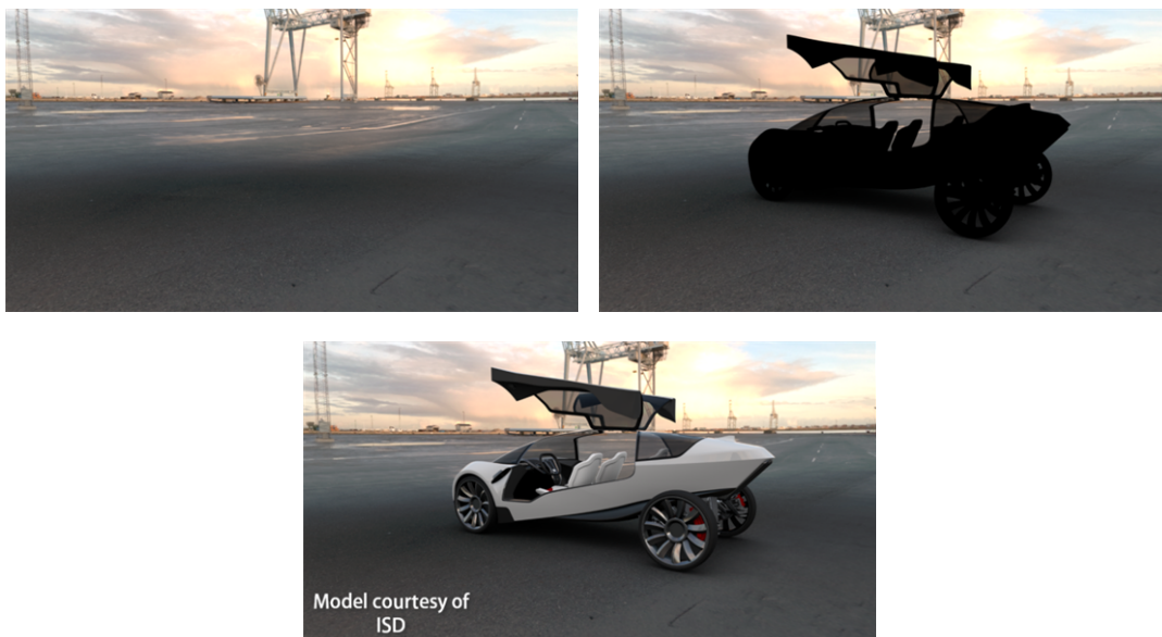
Figure 42 : Example of view reconstruction: over the background layer (left) the multiplicative layer (result of the process shown on the right) is applied. Then the additive layer is applied on the resulting view to reconstruct the final image (bottom).
