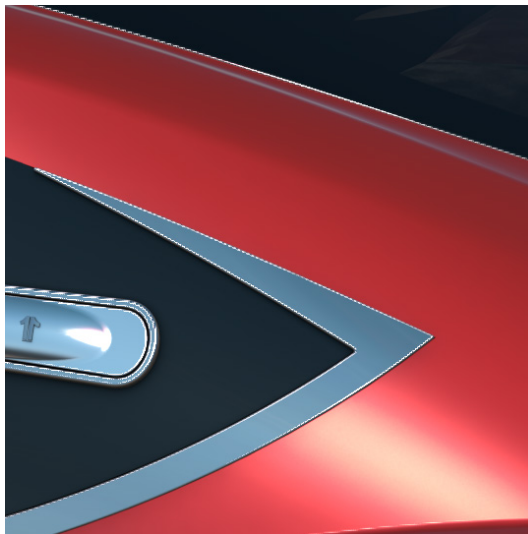
Figure 28 : Reflection of an environment featuring a high intensity area in a specular material without the High quality filtering option.
