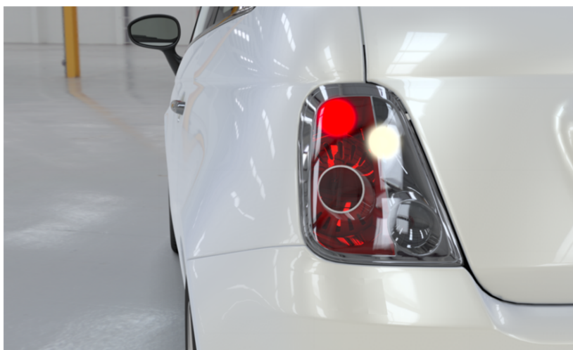
Figure 170 : Drago tone mapping with an average luminance of 0.5, a bias of 0.6 and a maximum input luminance of 1.
