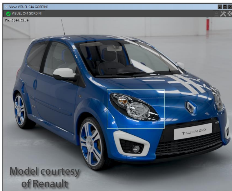
Raytracing rendering limited to a region of the view.
